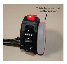
First, the switches have to be removed from the housing. Remove the main screws that hold the two housing halves together and gently open the two halves. Be careful to not stress or damage the wires that run between the two halves. Remove the insulating cover in the lower half over the starter switch and remove the strain relief.
