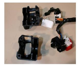
Now that the switches have all been removed from the housing, it is time to cut off the old throttle portion of the housing. The best method for cutting the housing is to use a band saw or table saw, but it is possible to cut it by hand using a hack saw if necessary. The most important part is to leave a little excess housing behind to be removed later, to avoid cutting into the switch part of the housing. This image illustrates where the cuts should go:
