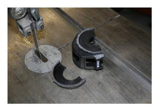
Once the excess housing is removed from both halves, the remaining part can be ground or filed off to complete the housing modification. We used a milling machine to remove the last part, but a file or a Dremel tool will work just as well.
