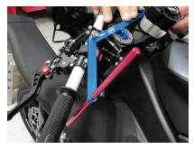
If you place the tool, and there is a space between the indicating rod and the handlebar, that means the handlebar is too far forward. Make adjustments to that handlebar, and check again with the tool. Move the tool to each side several times, and make adjustments as necessary to the sweep of the handlebars.
