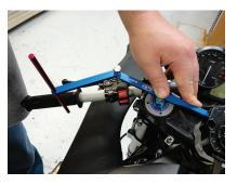
When the indicating rod lightly contacts both sides evenly, your handlebars are adjusted properly with identical sweep on both sides.
