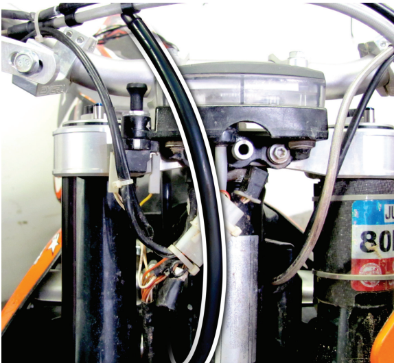
RIGHT SIDE T3 CABLE ROUTING.
