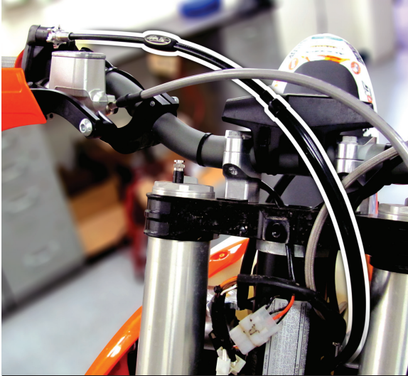
LEFT SIDE T3 CABLE ROUTING.
