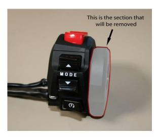
First, the switches have to be removed from the housing. Remove the main screws that hold the two housing halves together and gently open the two halves. Be careful to not stress or damage the wires that run between the two halves. Remove the insulating cover in the lower half over the starter switch and remove the strain relief.
