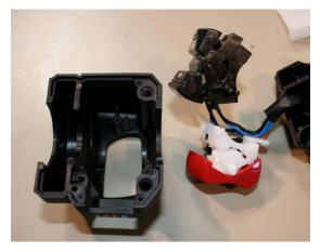
Next, clip the zip tie holding the wiring harness to the housing, and remove the starter button assembly from the housing. Be careful not to cut the sheath or any wires when cutting the cable tie. Remove the switch assembly from the lower housing.
