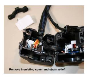
Pay attention to the routing of the wires, so that you can properly reassemble the switch when the housing modification is complete. Then remove the three screws in the upper half to remove the mode switch and engine kill switch.
