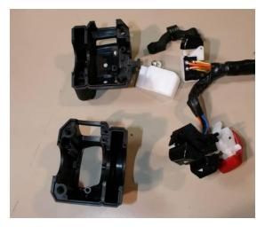
Now that the switches have all been removed from the housing, it is time to cut off the old throttle portion of the housing. The best method for cutting the housing is to use a band saw or table saw, but it is possible to cut it by hand using a hack saw if necessary. The most important part is to leave a little excess housing behind to be removed later, to avoid cutting into the switch part of the housing. This image illustrates where the cuts should go:
