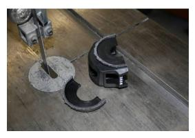
Once the excess housing is removed from both halves, the remaining part can be ground or filed off to complete the housing modification. We used a milling machine to remove the last part, but a file or a Dremel tool will work just as well.
