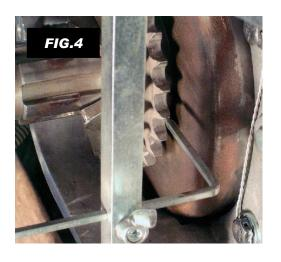
Rotate the tool 180 degrees and check the alignment of the pointer on a tooth of the motor sprocket. If the pointer is not in the middle of the tooth, adjust the thickness of the motor sprocket shim accordingly and repeat steps 1 and 2 (Fig. 3 & 4).
