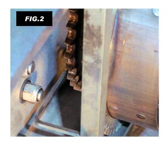
1. Hold the square bar against the inner primary cover and align the pointer with the middle of a tooth on the clutch shell, tighten thumb screw (Fig. 1 & 2).
